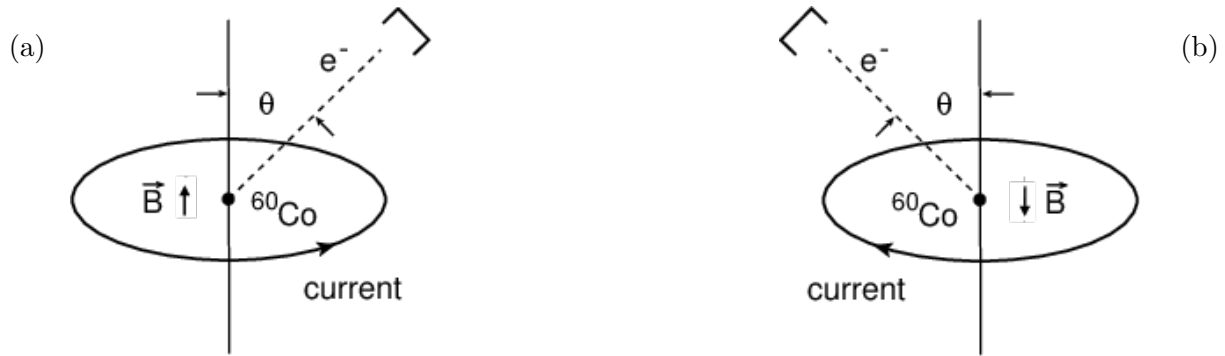
Figure 8.5: (a) An experiment in which nuclear spins are aligned parallel to a magnetic field created by a current loop, and the number of beta electrons is measured at the angle \theta . (b) The mirror image experiment.
