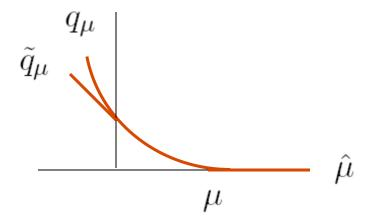
$$\tilde{q}_{\mu} = \begin{cases} \frac{\mu^2}{\sigma^2} - \frac{2\mu\hat{\mu}}{\sigma^2} & \hat{\mu} < 0\\ \frac{(\mu - \hat{\mu})^2}{\sigma^2} & 0 \le \hat{\mu} \le \mu\\ 0 & \hat{\mu} > \mu \end{cases}$$
