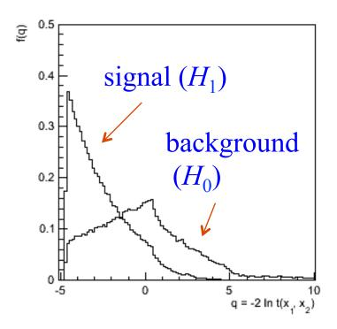
From the Neyman-Pearson lemma we know that by cutting on this variable we would select a signal sample with the highest signal efficiency (test power) for a given background efficiency.
