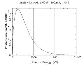
Figure 1: A photon energy spectrum from a synchrotron radiation source.
