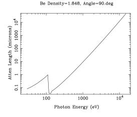
Figure 2: Attenuation length for x-rays in beryllium as a function of energy.
