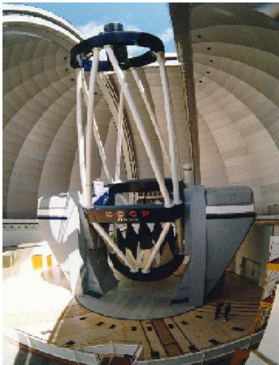
Figure 3.19: The 6-metre BTA (Bol'shoi Teleskop Azimutal'ny) or 'Large Azimuthal Telescope' on Mt. Pastukhov, Russia. This was the first large telescope to employ an alt-az mount [25].
