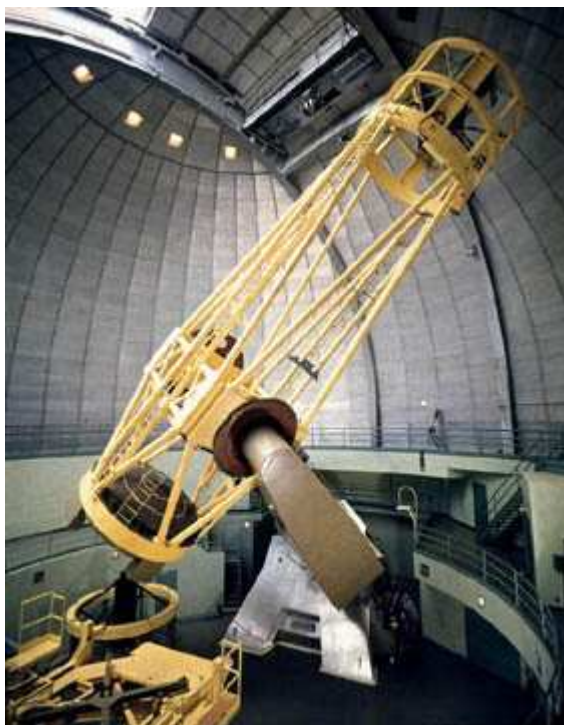
Figure 3.18: An example of an equatorial mount: the 3-metre diameter Shane Telescope at the Lick Observatory, California [24].
