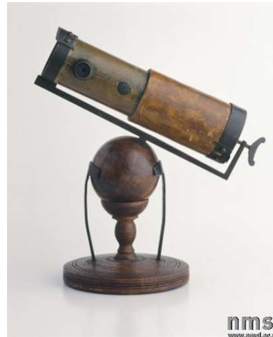
Figure 3.7: (a) Illustration of the focal length for a reflecting telescope. (b) Replica of Newton's original reflector (total length approx. 7 inches) [12].
