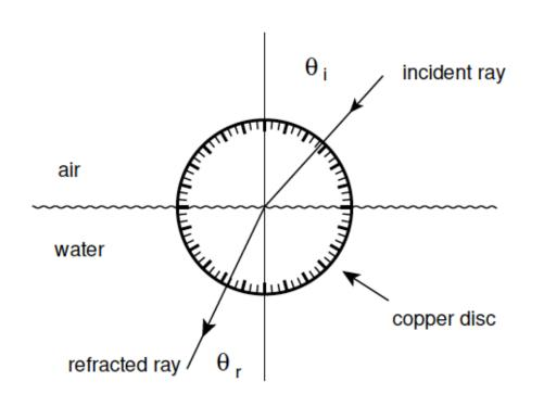
Angles of incidence and refraction (degrees)
