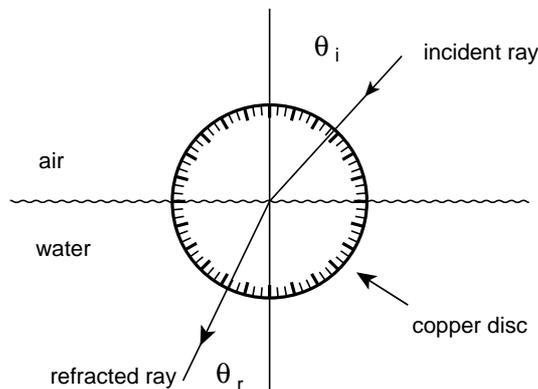
Figure 7.2: The apparatus used by Ptolemy to investigate the refraction of light.
