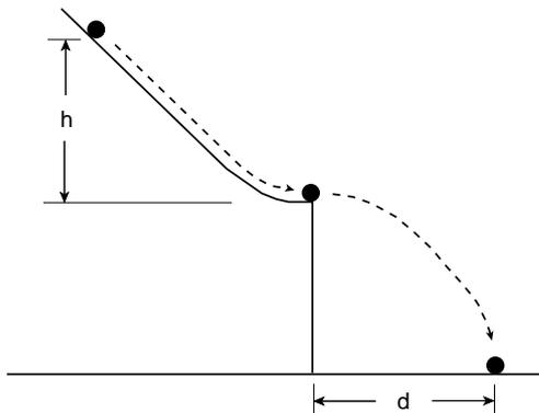
Figure 7.1: The configuration of the ball and ramp experiment performed by Galileo.
