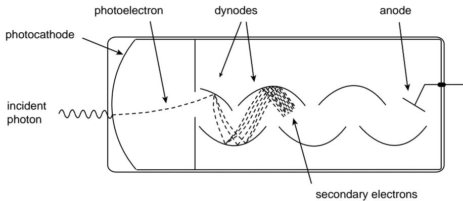
Figure 3.1: Schematic drawing of a photomultiplier tube.
