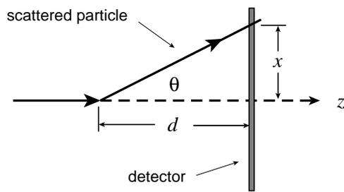
Figure 9.1: The definition of the scattering angle  $\theta$  from the trajectory projected into the  $(x, z)$  plane.
