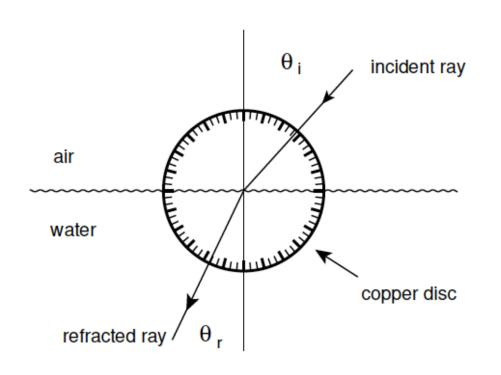
Angles of incidence and refraction (degrees)
