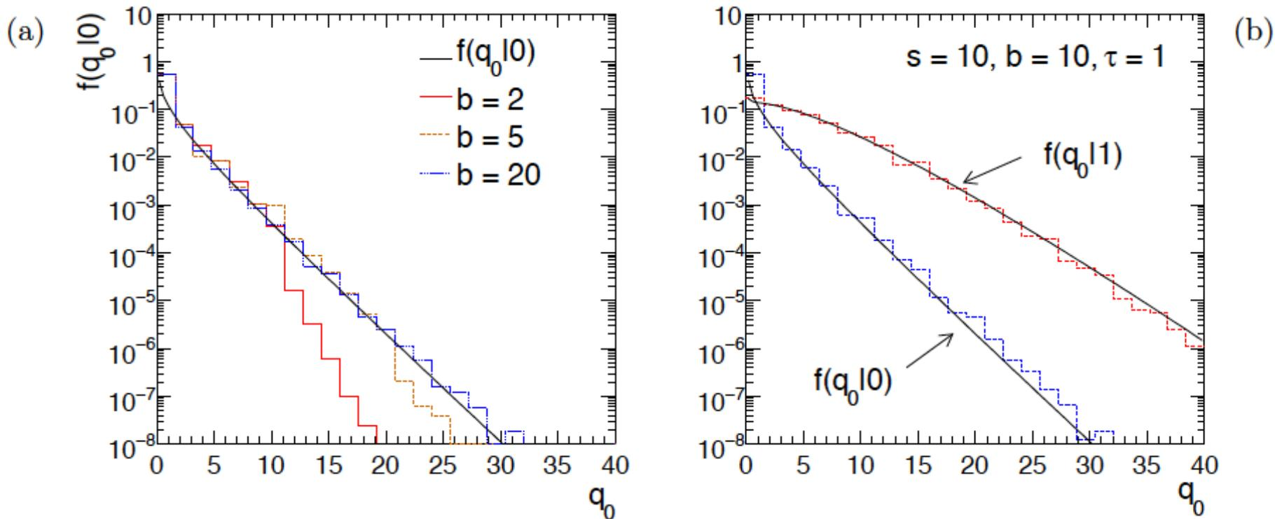
Figure 3: (a) The pdf  $f(q_0|0)$  for the counting experiment. The solid curve shows  $f(q_0|0)$  from Eq. (49) and the histograms are from Monte Carlo using different values of  $b$  (see text). (b) The distributions  $f(q_0|0)$  and  $f(q_0|1)$  from both the asymptotic formulae and Monte Carlo simulation based on  $s=10$ ,  $b=10$ ,  $\tau=1$ .
