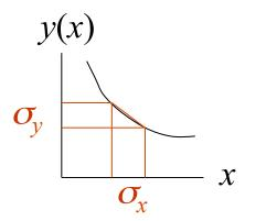
Limitations: exact only if  $\vec{y}(\vec{x})$  linear. Approximation breaks down if function nonlinear over a region comparable in size to the  $\sigma_i$ .
