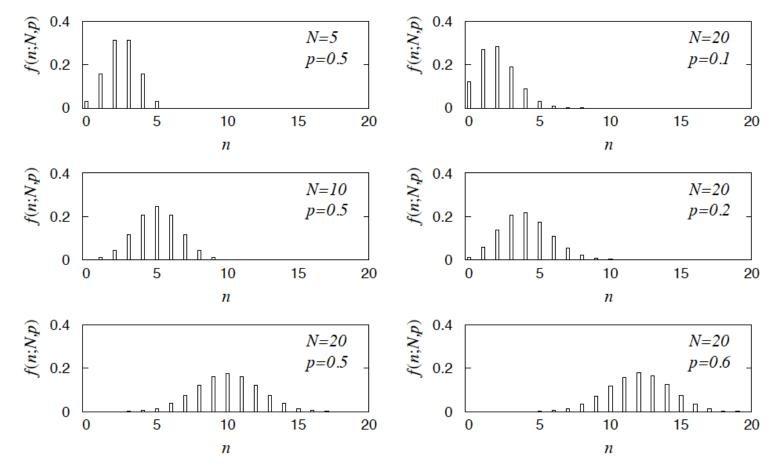
Example: observe *N* decays of  $W^{\pm}$ , the number *n* of which are  $W \rightarrow \mu \nu$  is a binomial r.v., *p* = branching ratio.
