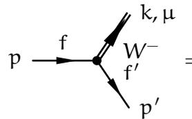
$$= -i \frac{g}{\sqrt{2}} V_{ff'} \tau^+ \gamma_\mu \frac{1 - \gamma_5}{2} \quad (178)$$
