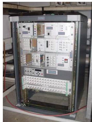
Fig. 5.3 The electronics designed and built at RHUL to control the laser-wire scanning and diagnostics. This now sits in the PETRA tunnel.
