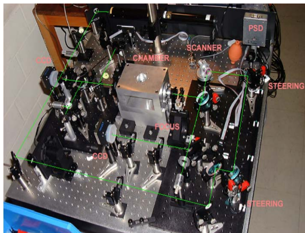
Fig. 5.2 The steering and laser diagnostics set-up at RHUL before shipment to DESY. The test vacuum vessel (centre) was also made at RHUL.
