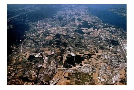
Detectors at 4 pp collision points: ATLAS CMS general purpose LHCb (b physics) ALICE (heavy ion physics) Counter-rotating proton beams in 27 km circumference ring
