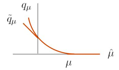
$$\tilde{q}_{\mu} = \begin{cases} \frac{\mu^2}{\sigma^2} - \frac{2\mu\hat{\mu}}{\sigma^2} & \hat{\mu} < 0\\ \frac{(\mu - \hat{\mu})^2}{\sigma^2} & 0 \le \hat{\mu} \le \mu\\ 0 & \hat{\mu} > \mu \end{cases},$$
